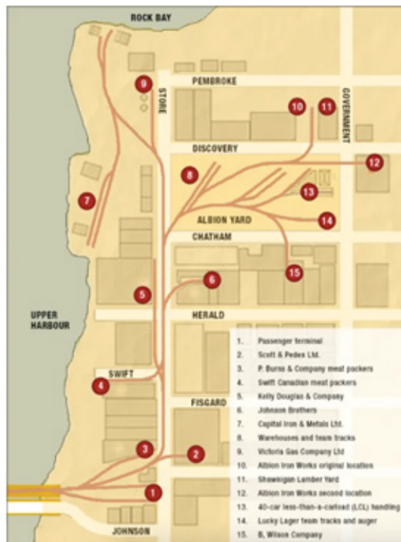
Map by Denton Pendergast The rail plan of the Esquimalt and Nanaimo's Victoria rail service.
