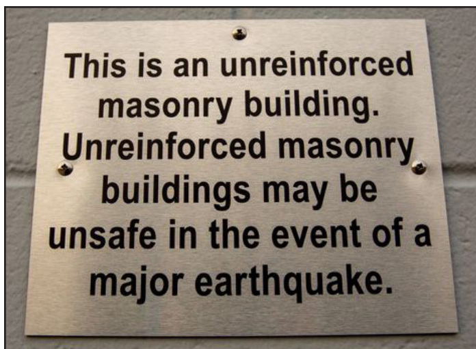
Fig. 4.3: Example of a seismic hazard sign installed on URM buildings in California. (Source: Courtney Sherwood)
