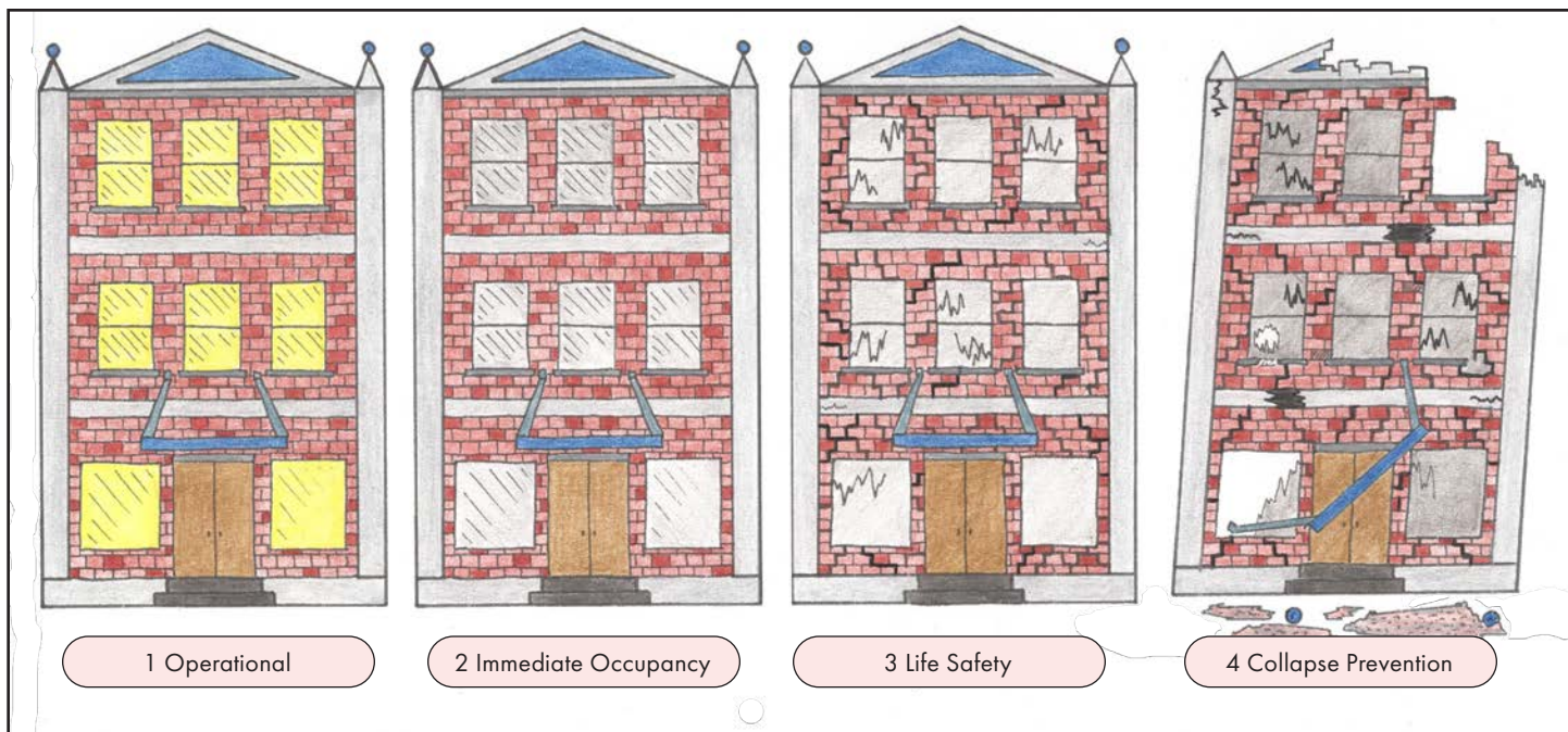
Fig. 3.2: Illustration of the different building performance levels that heritage buildings can be seismically upgraded to. (Source: Ian Babbitt, based on the American Society of Civil Engineers performance level illustration from ASCE 41)
