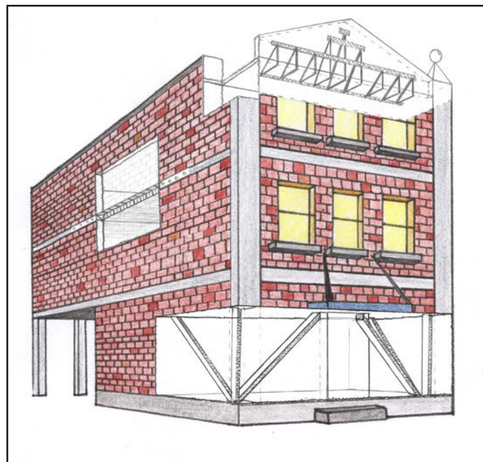
Fig. 3.3: Illustration of some of the different seismic upgrading options available. (Source: Ian Babbitt)
