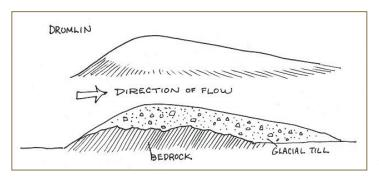
Figure 25: Schematic illustration of how drumlins form when glacial ice moves over unconsolidated sediments.
